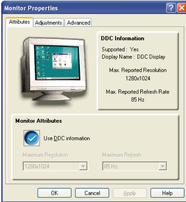
DDC is the technology whereby the monitor communicates to the graphics card all the resolutions and refresh rates it supports. The RADEON™ family of graphics cards are all DDC compliant.
